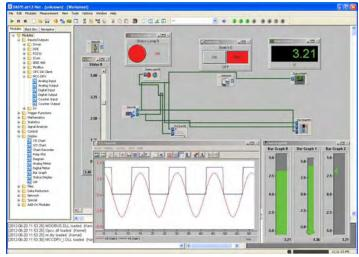
DASYLab gives users the ability to create applications by simply dragging-and-dropping functional icons on a worksheet, connecting the icons together, and running the program. DASYLab supports most data acquisition hardware.
