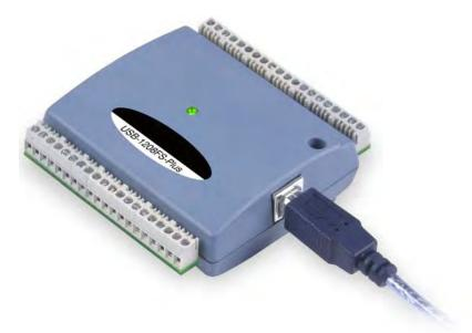
All devices in this series offer eight singled-ended or four differential analog inputs, two analog outputs, 16 digital I/O, and one counter input. The USB-1208FS-Plus/1408FS-Plus also include eight high-current (24 mA) digital I/O connections and DAQFlex support.
