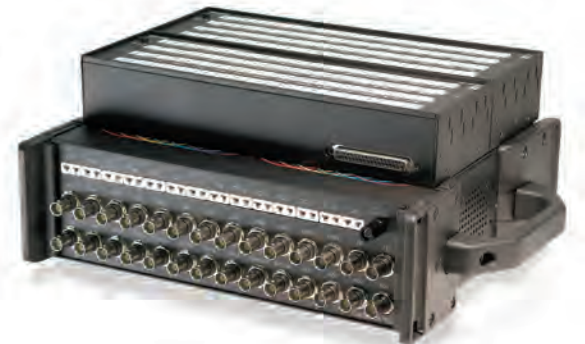
DaqBook/2000 system plus 112 additional channels of thermocouple input (DBK90)
