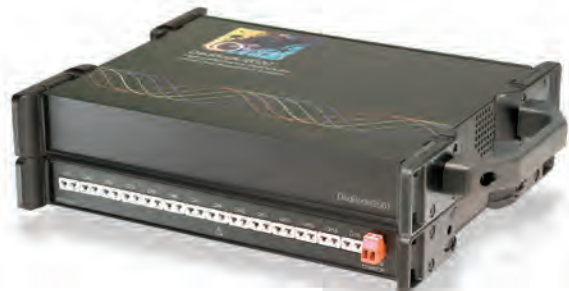
DaqBook/2001 plus 14 channels of thermocouple inputs (DBK84)
