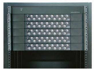
The 80 channel high-speed scanning system consists of one DaqScan/2005 plus five DBK85 16-channel voltage scanning modules. All channels can be measured at the maximum rate of 5 µs/channel.
