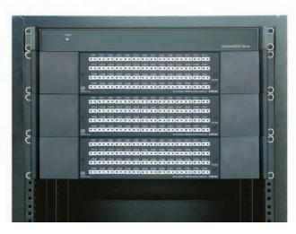
The 168 TC channel system consists of one DaqScan/2005 plus three DBK90 modules with rack-mount kits
