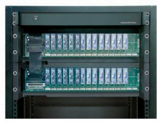
The 32-channel isolated system includes a DaqScan/2005 plus two DBK207/CJC boards. The system is capable of scanning all channels at 5 µsec per channel, and provides 500V isolation for all inputs.
