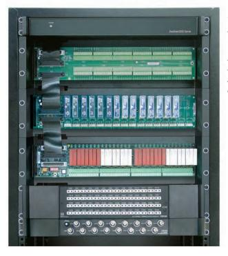
The system provides 56 non-isolated TC inputs, 16 isolated voltage inputs, 16 low-voltage inputs, 4 analog outputs, 4 frequency inputs, and 32 isolated discrete high-voltage outputs
