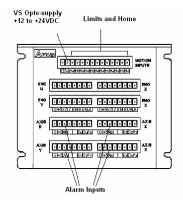
Note: Limit/Home input pins are identical for both standard as well as DB9 top board.
