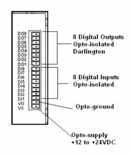
Note: Digital inputs and outputs are found on the bottom board of the PMX-4EX-SA.
