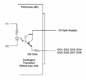
For the opto-isolated outputs, the digital output signal will source from the VS optosupply when the signal is turned on.
