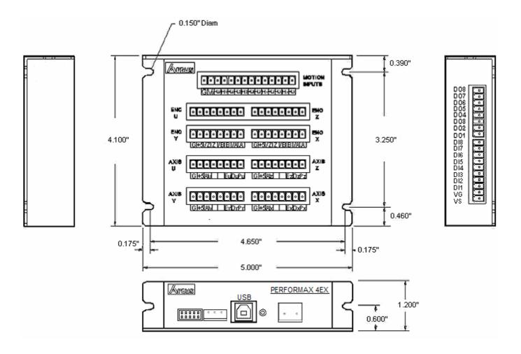
Note: The image above is of PMX-4EX-SA-TBS. The dimensions of PMX-4EX-SA-TB9 are the same, with the exception of the top board connectors.
