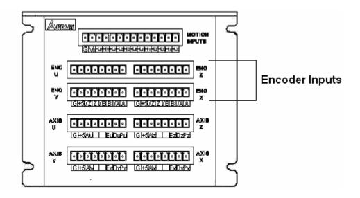
Note: Encoder pins are identical for both standard as well as DB9 top board
