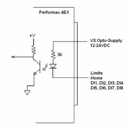
To trigger the opto-isolated digital inputs, sink the digital input signal to the ground of the VS.
