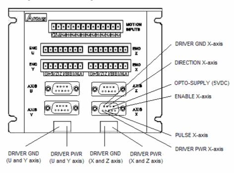
The pins on the DB9 headers can be connected directly to a DMX-A2-DRV module (pinto-pin compatible)
