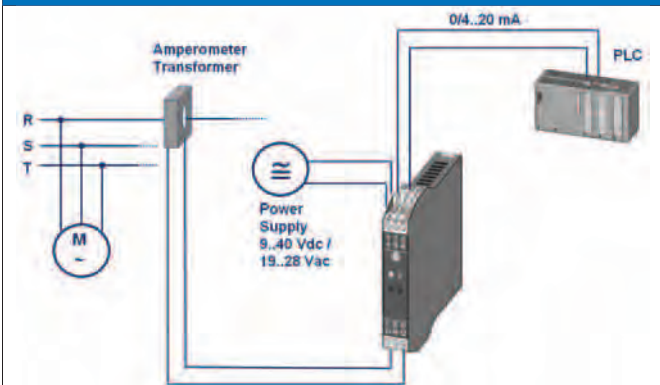
Z201 – AC current to DC converter / isolator
