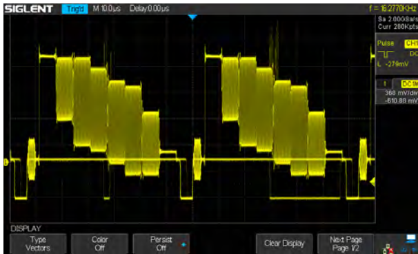
256-level intensity grading display on waveform
