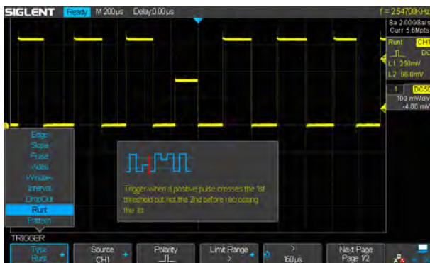
Edge, Slope, Pulse, Video, Windows, Runt, Interval, Dropout, Pattern, IIC, SPI, UART/RS232, LIN and CAN
