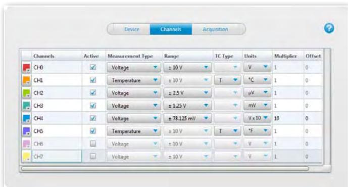
Use the channels grid to activate and configure channels to include in an acquisition. DAQami can acquire voltage and temperature data, and includes options for input range, thermocouple type, and units. Users can also create custom units with a configured multiplier and offset.
