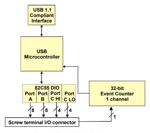
Figure 1-2. USB-1024LS functional block diagram
