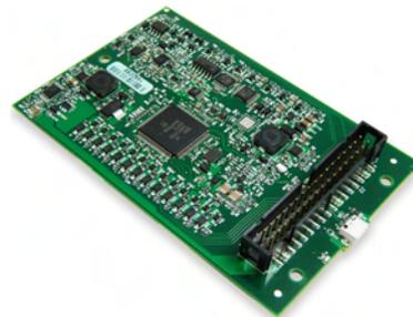
*The OEM versions have the same specifications as the standard devices, but come in a board-only form factor with a header connector instead of screw terminals.*
