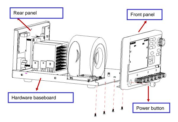
**Step 5: Remove the front panel components**
