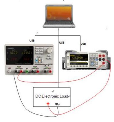
2. Double click and run the script **CurrentCalib.py** prepared previously. Then Change the channel connection according to the prompt message.
