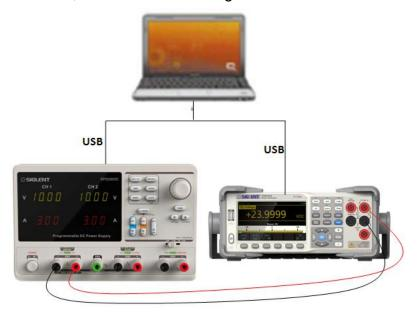
2. Double click and run the script VoltageCalib.py prepared previously. Then Change the channel connection according to the prompt message.
