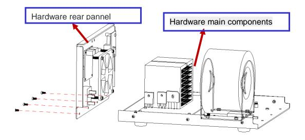
**Step 7: Remove hardware rear pannel components**
