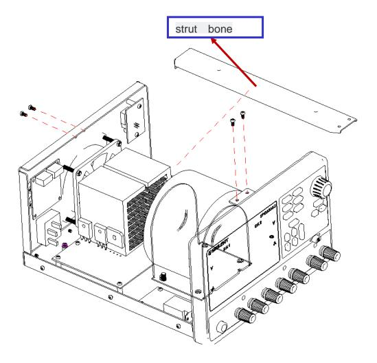
**Step 4: Separate the front panel and the hardware components**
