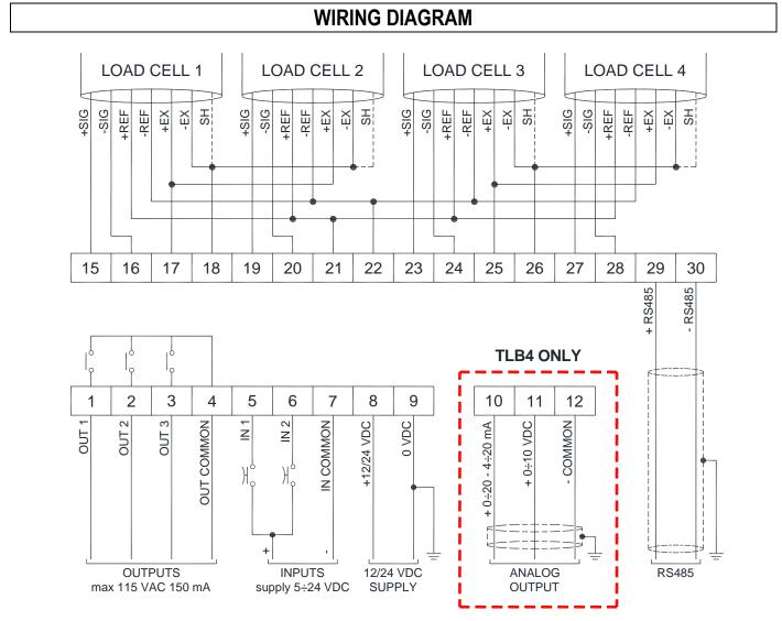
In case of difficulty connecting all the reference wires of the installed load cells, simply connect those of the load cell located at the average distance from the instrument. The reference wires not used must be individually isolated.
