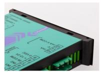
Pull out the terminal strips and insert the instrument into the hole.
