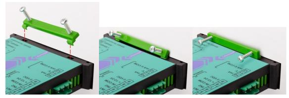
Insert the mounting brackets into the housings, on both sides of the instrument.
