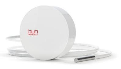
message alarms as soon as temperature exceeds or falls below pre-set limits. It also provides access to the records history, graphs and periodical reports. Its hardware and software installation is very easy and does not require any specific tools or applications.
