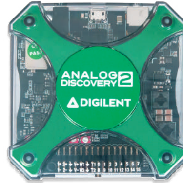
Analog Discovery 2: 100MS/s USB Oscilloscope, logic analyzer and variable power supply
