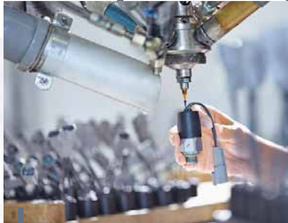
Encapsulating system for custom ready-wired pressure switches for strictest requirements of IP protection class.
