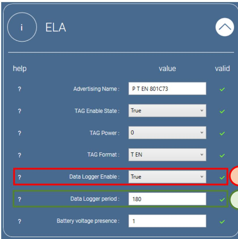
To use the data logger, you must set the **Data Logger Enable** field to **True**. (1)
