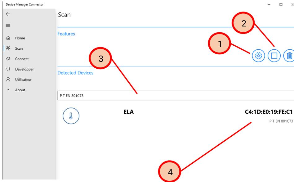
Simply click on a tag in the list to connect to that tag. The application then switches to the connection screen, which displays all the information and available commands for the selected tag.
