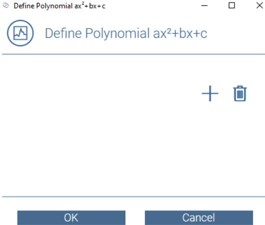
You can add a calibration coefficient by clicking on the **+** button. You can add up to 3 coefficients.
