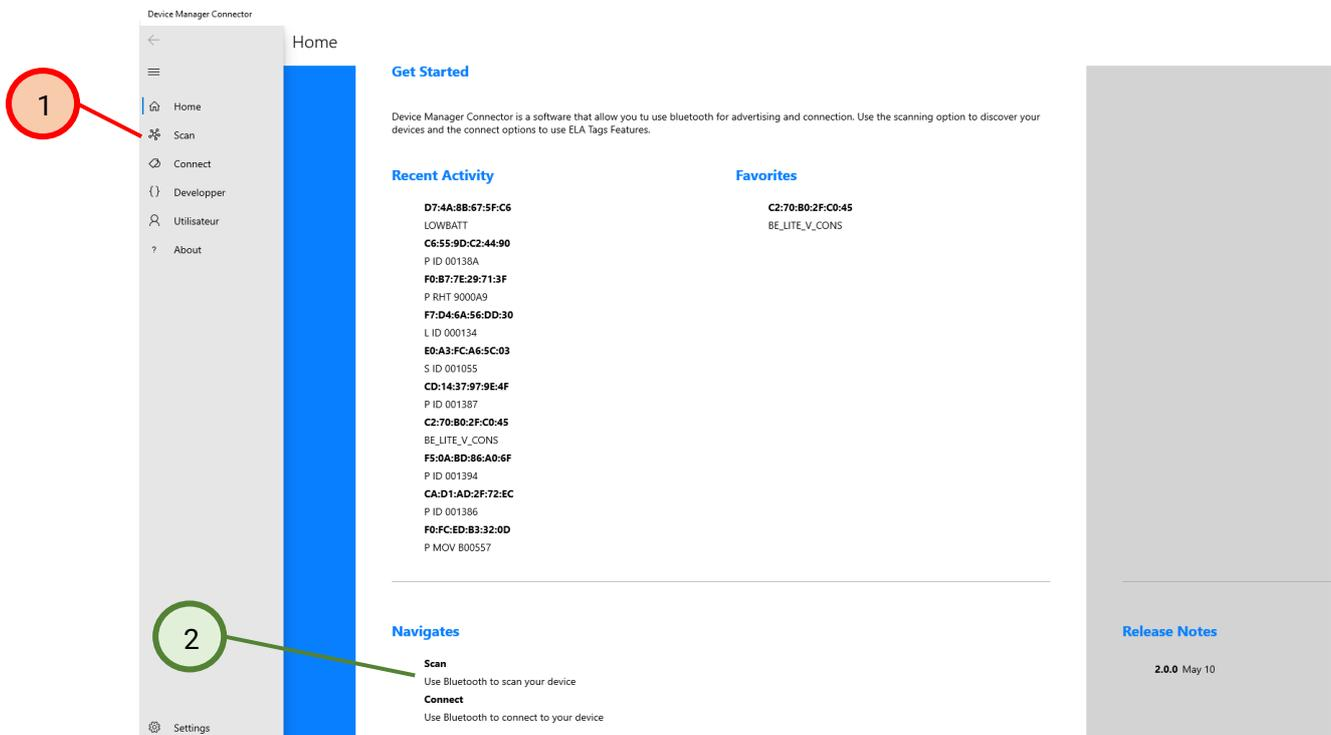
With the Scanner function, you can start “listening” for Bluetooth communications by clicking on the Bluetooth Scan button. At any time, you may define a filter to more precisely target the tag that you want to access. The search bar enables you to browse through all the detected tags and refine your selection based on MAC address, tag name, etc.
