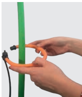
First generation Rogowski sensor, output 100 mV/kA, 50-60 Hz, Ø 115 mm
