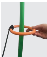
RC-V250-100 First generation Rogowski sensor, output 100 mV/kA, 50-60 Hz, Ø 115 mm
